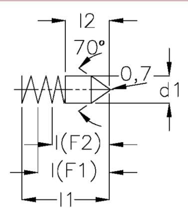
$\begin{array}{lll} \text{d1} & = 2.2 \\ \text{I(F1)} & = 12.0 \\ \text{I(F2)} & = 10.5 \\ \text{I1} & = 16 \\ \text{I2} & = 7.8 \\ \text{Spring pressure (F1) N = 2.2} \\ \text{Spring pressure (F2) N = 3.0} \end{array}$
